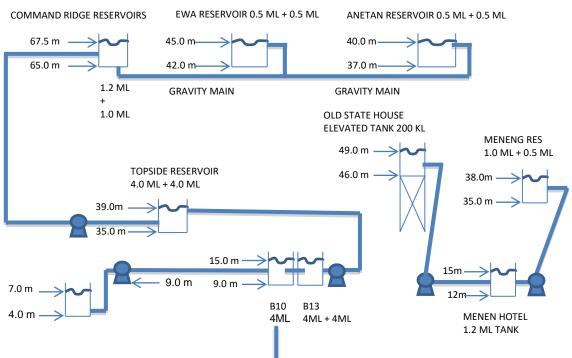
Figure 43. The Original 2035 schematic on which system analysis was based.
