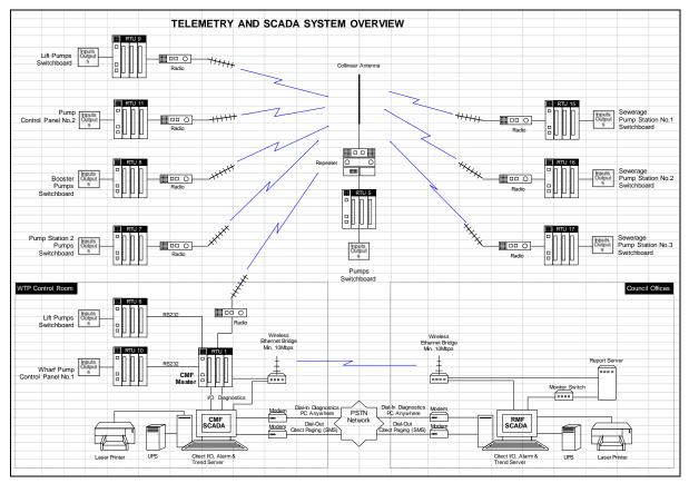
Figure 109. Example of Telemetry and SCADA system
