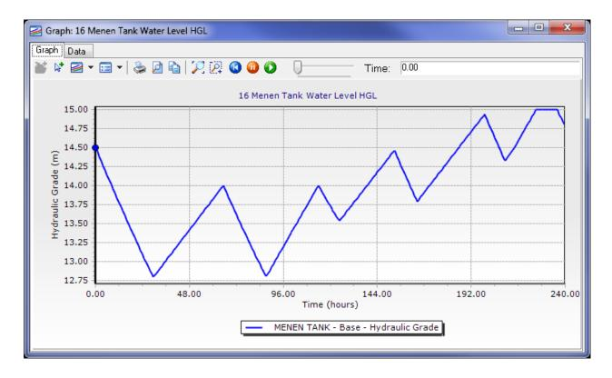
Figure 80. Menen Desalination Plant Tank Level (HGL)
