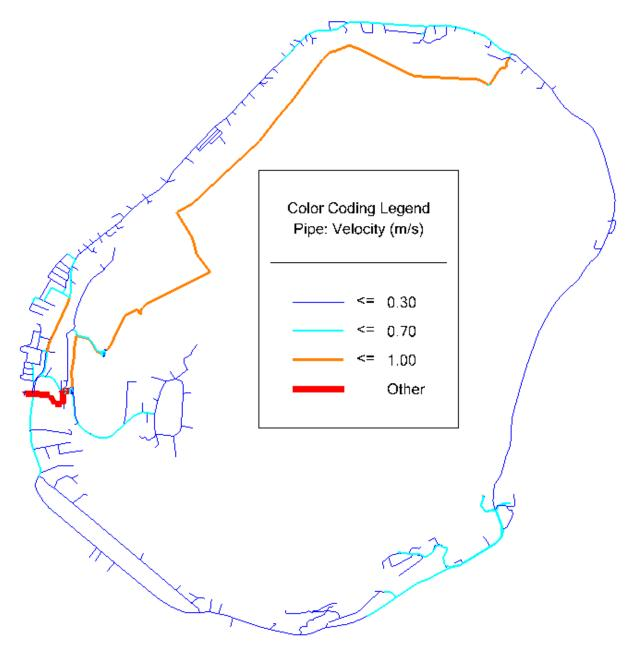
Figure 90. Pipe velocities at 8 am peak flow on day 1
