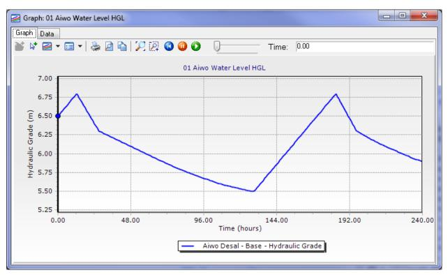
Figure 65. Aiwo Desalination Plant Tank Water Level (HGL)
