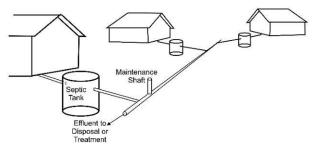
Figure 94. Schematic of CED System
