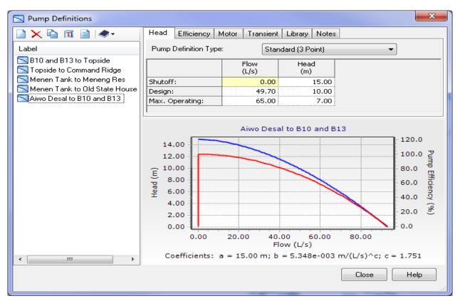
Figure 58. Pump Curve – Aiwo Desal to B10 and B13
