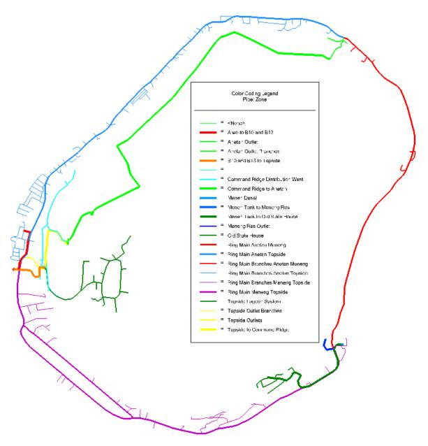
**Figure 60. Zones** Figure 60 shows the pipework in the WaterGEMS model colour coded by zone.
