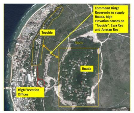
Figure 40. Supply Area from Command Ridge Reservoirs
