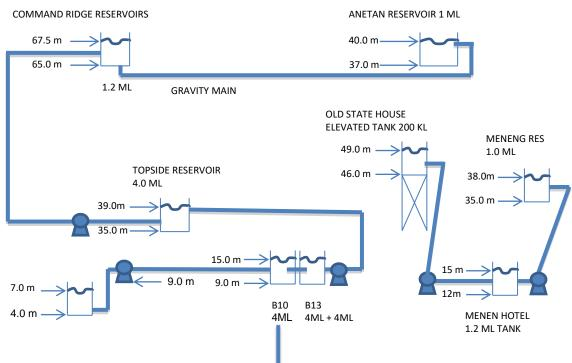
Figure 107. Final 2025 Phase 1 Water Supp y Schematic.
