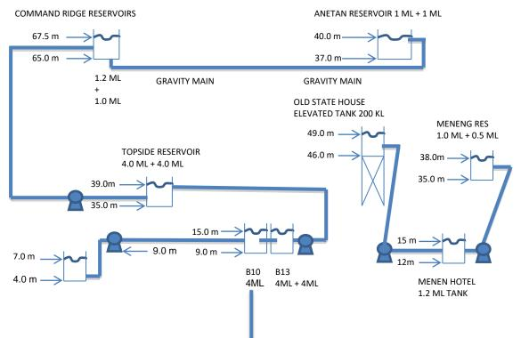
Figure 108. Final 2035 Phase 1 Plus Phase 2 Water Supply Schematic.
