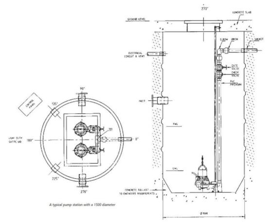
Figure 100. Detail of Prefabricated Pump Station
