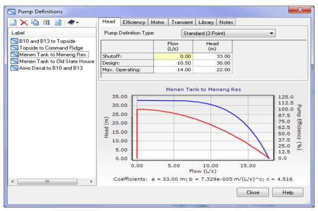
Figure 56. Pump Curve – Menen Tank to Meneng Reservoir
