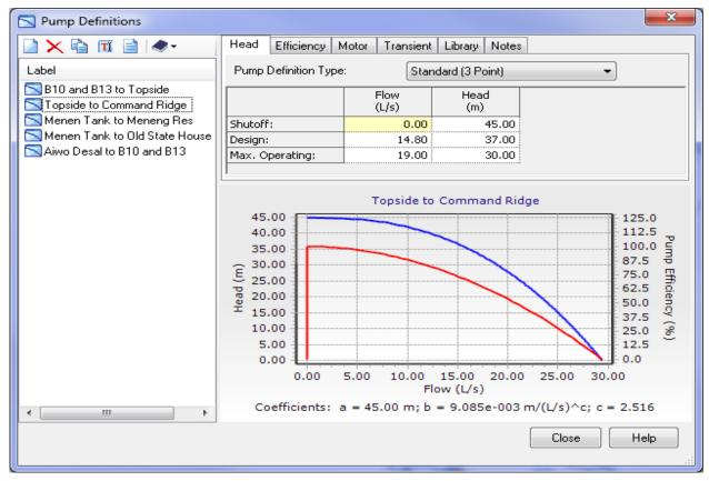
Figure 55. Pump Curve – Topside to Command Ridge
