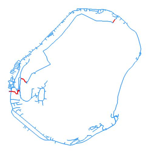
Figure 63. Ductile Iron pipework highlighted in red
