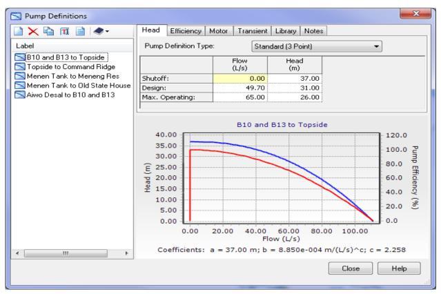
Figure 54. Pump Curve - B10 and B13 to Topside
