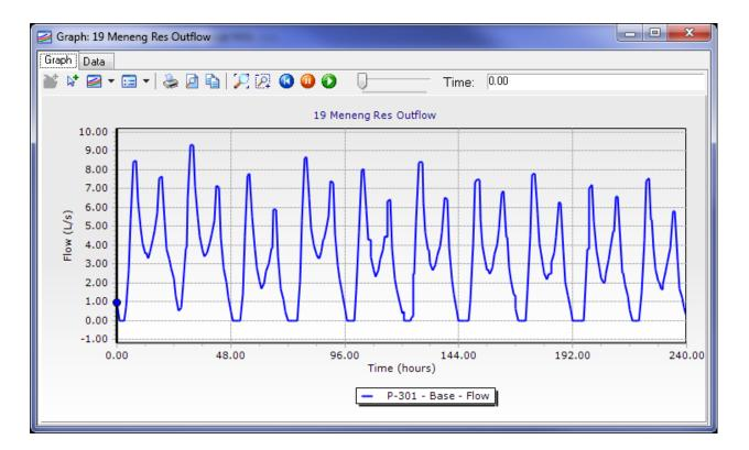
Figure 83. Meneng gravity flow to ring main
