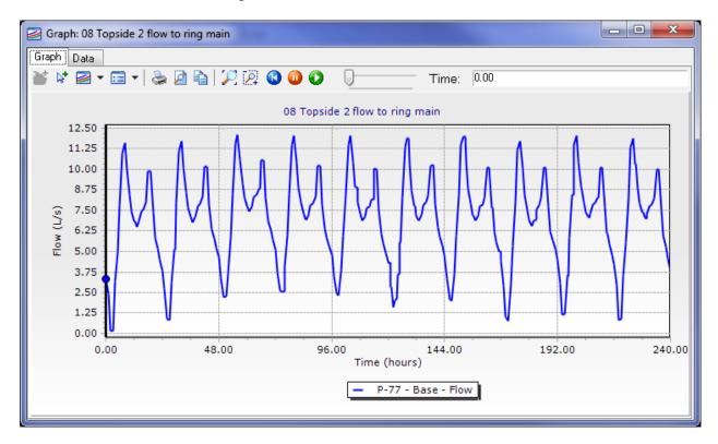
Figure 72. Topside Tank 2 gravity flow to ring main
