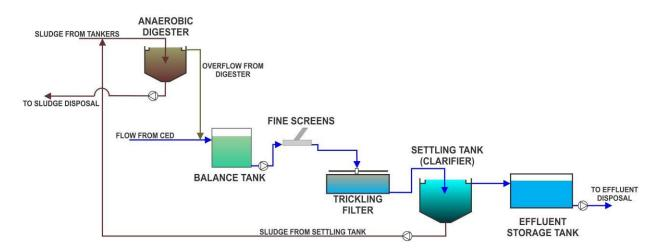
Figure 101. Municipal Treatment Plant Process Schematic
