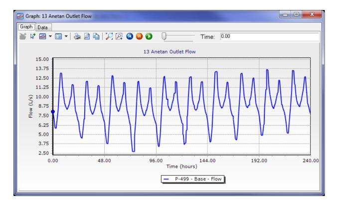
Figure 77. Anetan gravity flow to ring main
