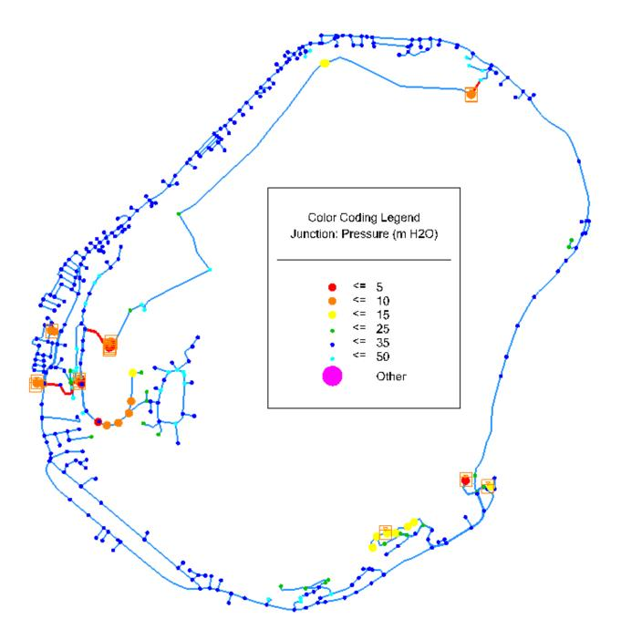
**Figure 88. Pressures at 3 am low flow on day 10** Figure 88 confirms that no pressures exceed 50 m.
