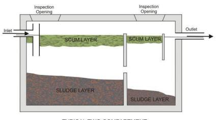
TYPICAL TWO COMPARTMENT SEPTIC TANK
