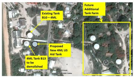
Figure 32. B10 and B13 Tank Farm
