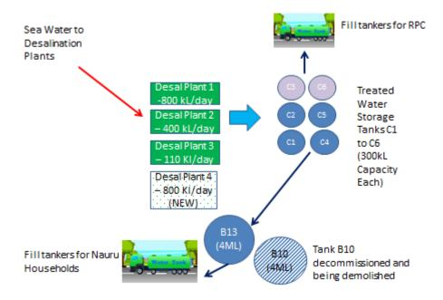
Figure 2. Current Water Supply System Operation
