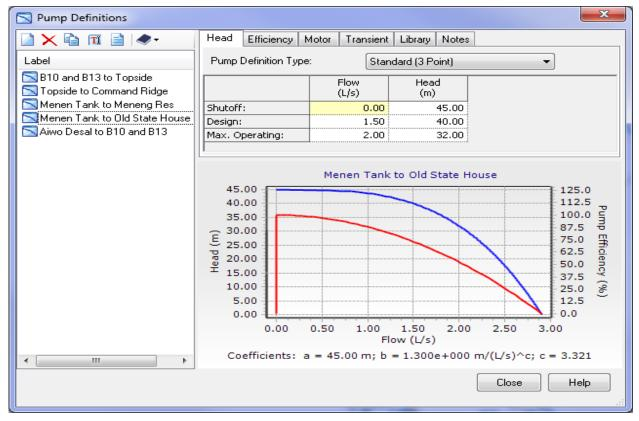
Figure 57. Pump Curve – Menen Tank to Old State House
