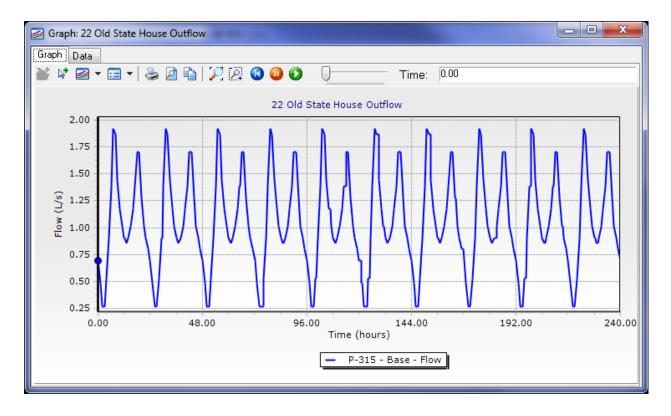
Figure 86. Old State House gravity flow to distribution
