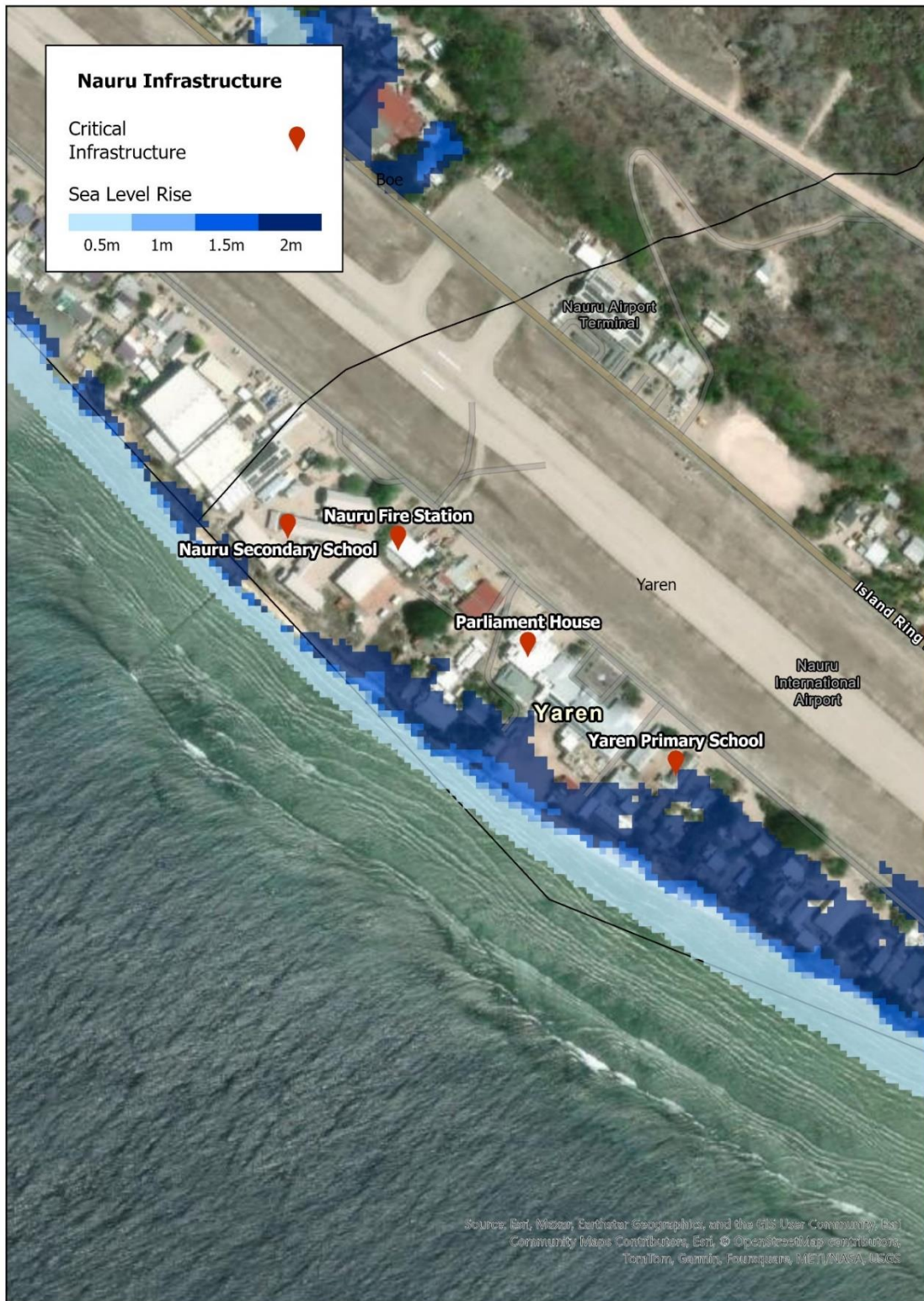
Figure 23 Yaren Critical Infrastructure Impacted by Sea Level Rise of 0.5, 1.0, 1.5, and 2.0 as indicated by the blue shaded areas (see image legend).
