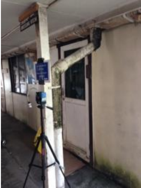
Photo 1 - Air Sample Pump on Tripod
