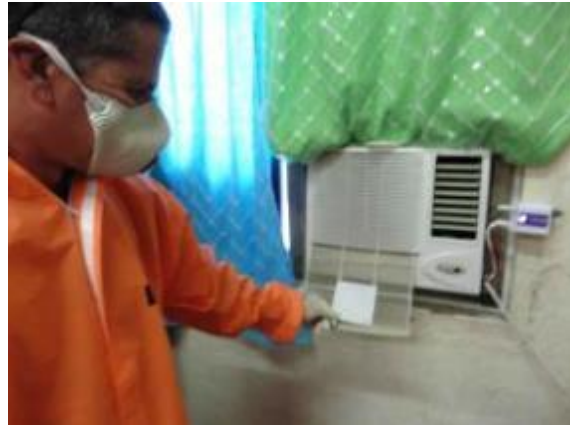
Photo 4 – Swab Sample of an Air-Conditioner
