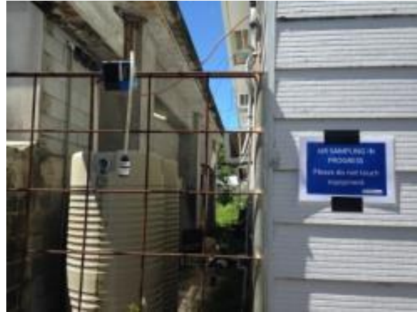
Photo 2 – Air Sample Pump on Fence
