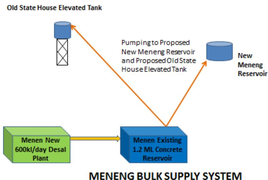
**Figure 26. Proposed Meneng Bulk Water Supply System**
