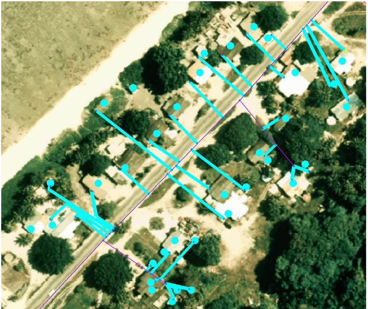
Figure 92. Sample customer connection pipework in northwest Nauru
