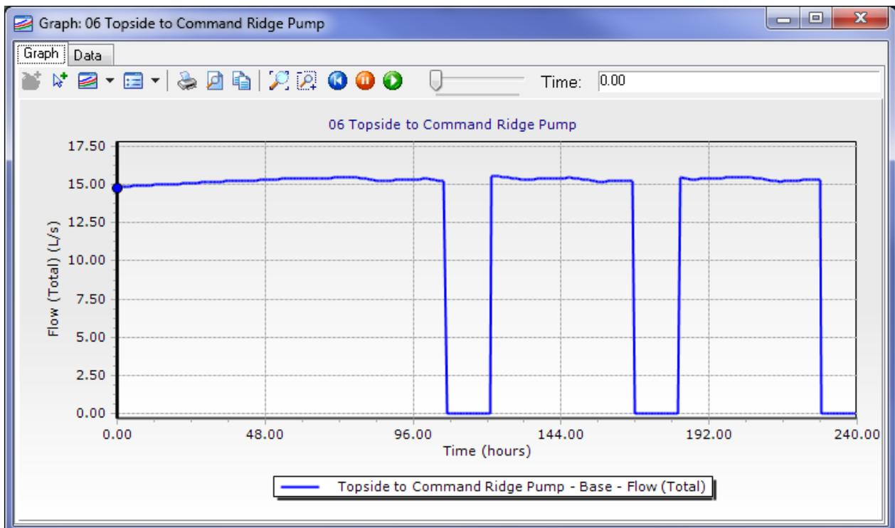
**Figure 70. Pumped Flow from Topside to Command Ridge**
