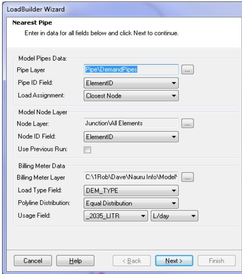
**Figure 51. WaterGEMS Loadbuilder was used to allocate demand seed points to pipes**
