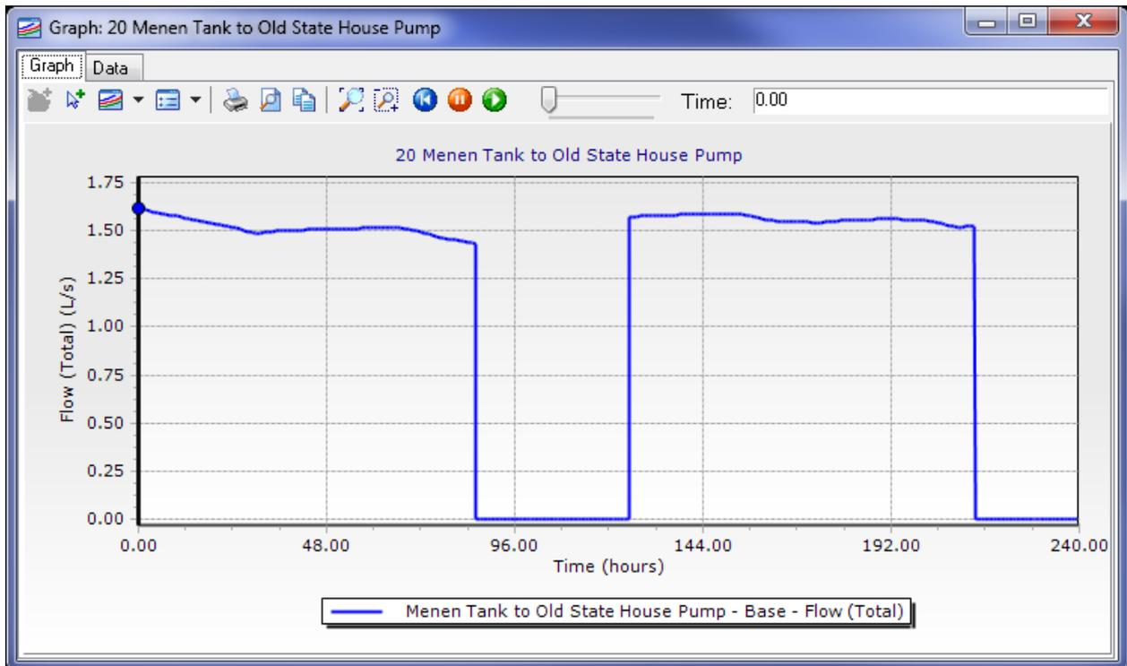
**Figure 84. Pumped flow from Menen to Old State House Water Tower**
