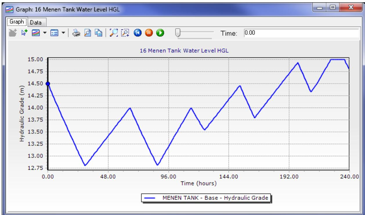
**Figure 80. Menen Desalination Plant Tank Level (HGL)**
