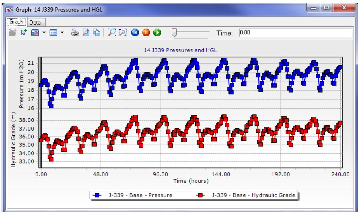
Figure 78. Pressures and HGL at one of the high spots between Topside and Meneng
