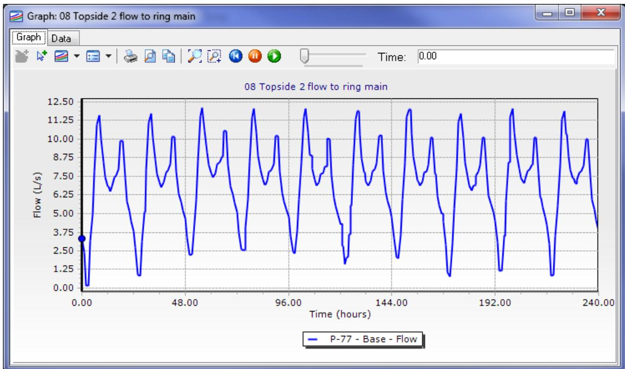
**Figure 72. Topside Tank 2 gravity flow to ring main**
