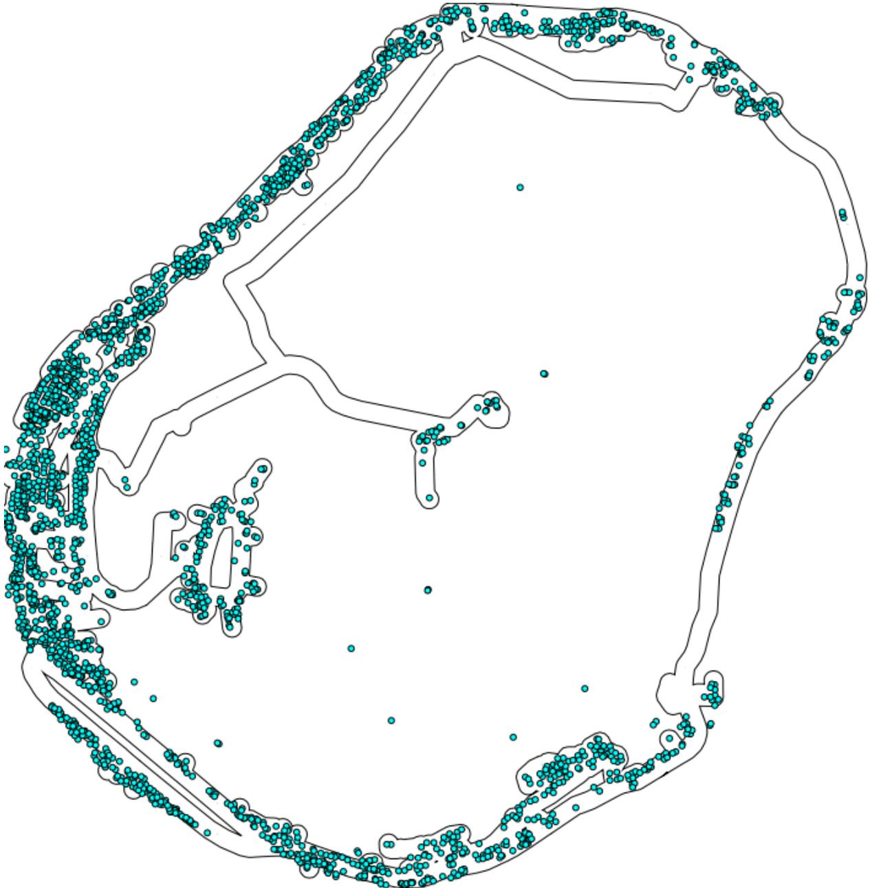
**Figure 46. Buffer proximity analysis of pipes to customer demand seed points**
