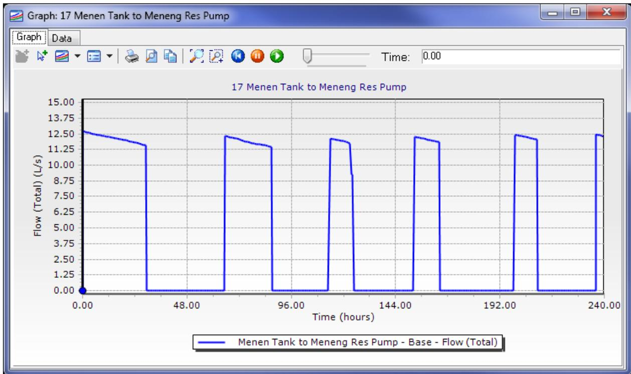
**Figure 81. Pumped flow from Menen to Meneng Tank**
