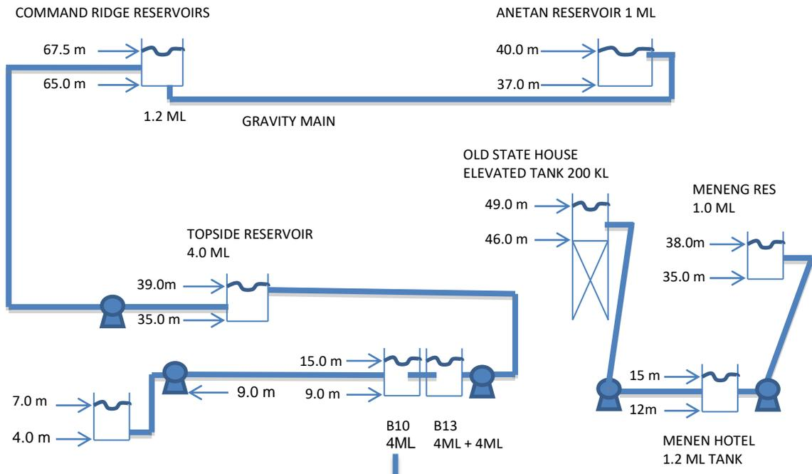
**Figure 107. Final 2025 Phase 1 Water Supply Schematic.**
