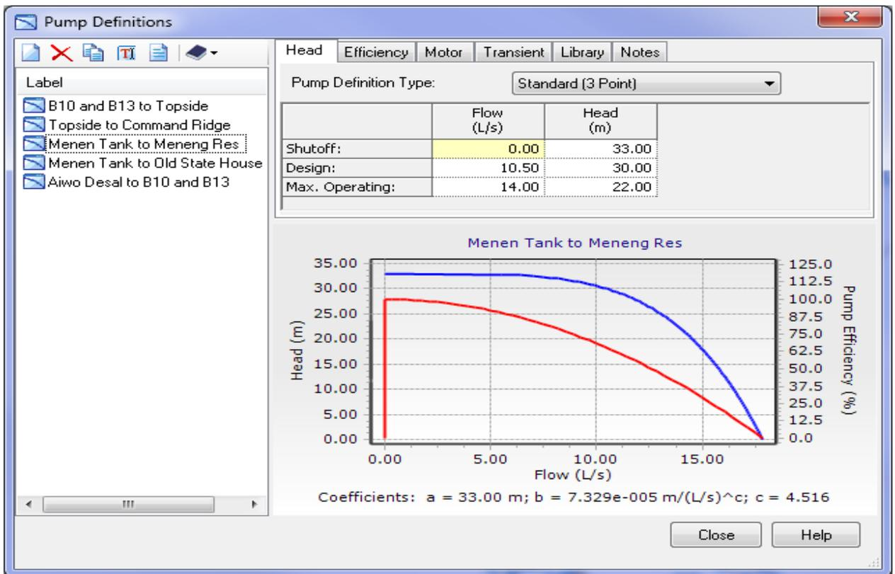
Figure 56. Pump Curve – Menen Tank to Meneng Reservoir
