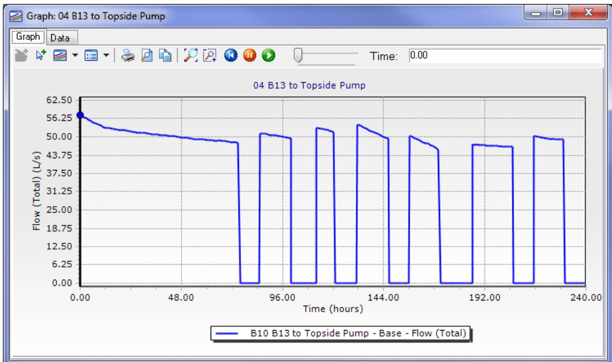
**Figure 68. Pumped flow from B10 and B13 to Topside**
