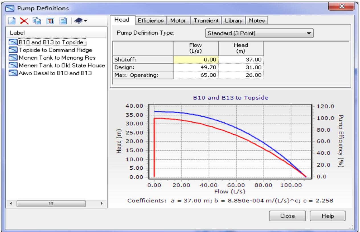
Figure 54. Pump Curve - B10 and B13 to Topside
