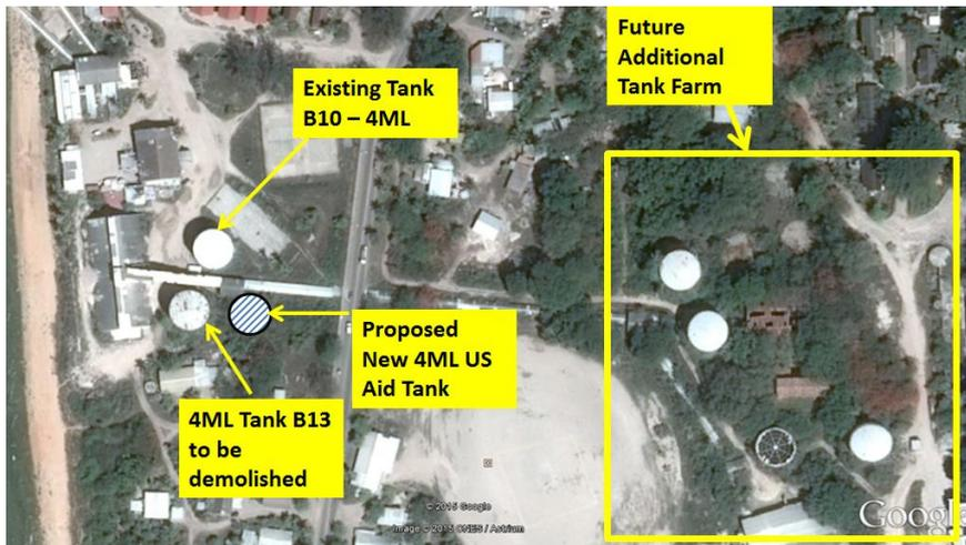
**Figure 32. B10 and B13 Tank Farm**
