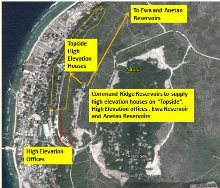
**Figure 24. Command Ridge Supply area**
