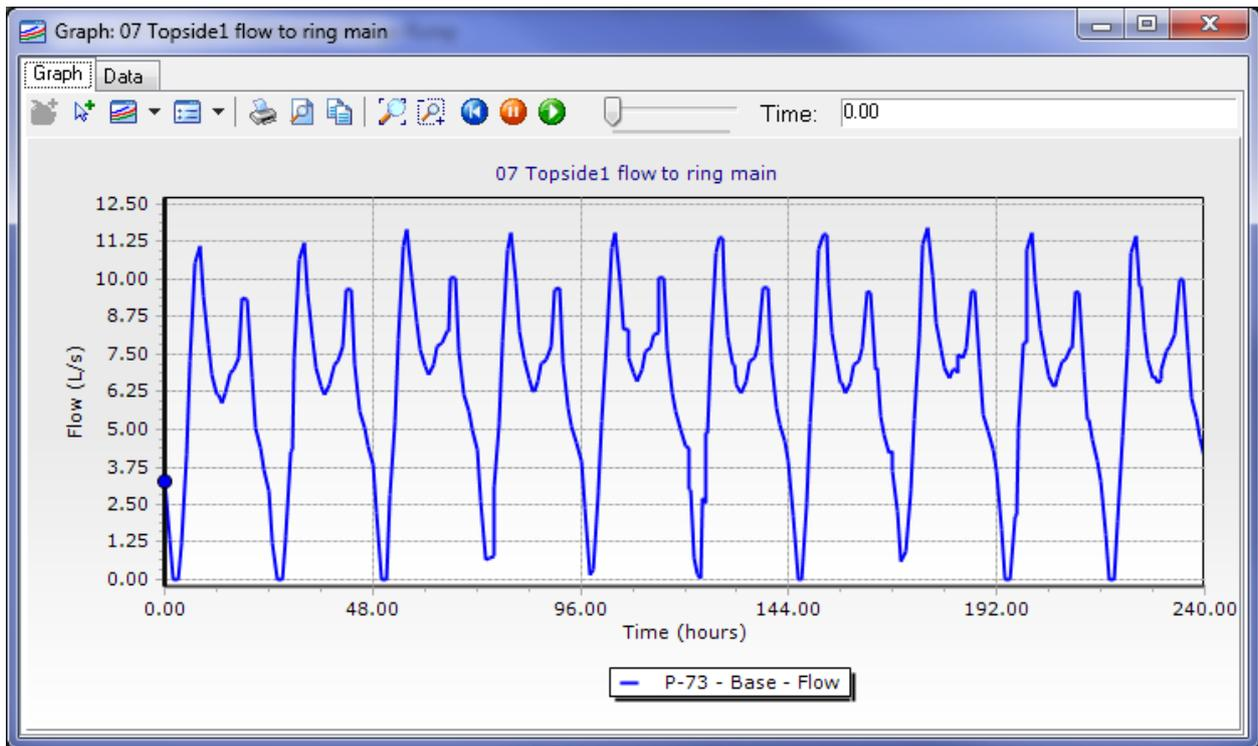
**Figure 71. Topside Tank 1 gravity flow to ring main**
