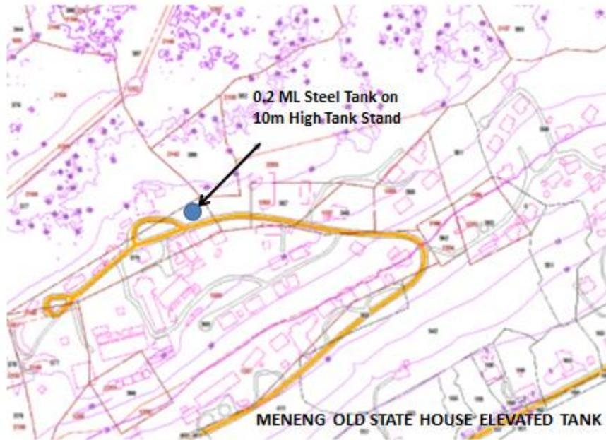
**Figure 39. Proposed Old State House Elevated Tank Location**
