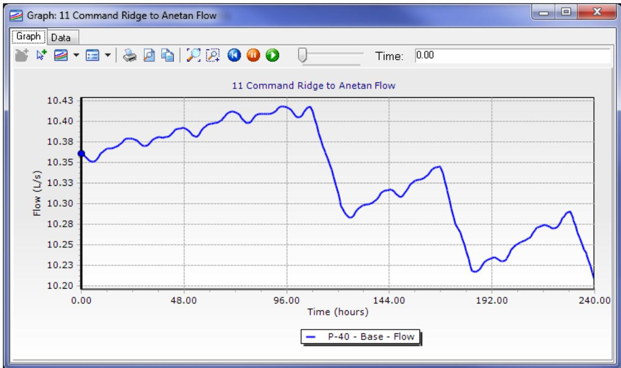
**Figure 75. Command Ridge gravity flow to Anetan Tanks**
